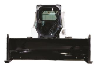
The Snow Pusher moves snow up to 5 times faster that a conventional snow blade. Available from 84" to 120" unit is designed for great visibility. The design features adjustable wear shoes and a high carbon cutting edge.
