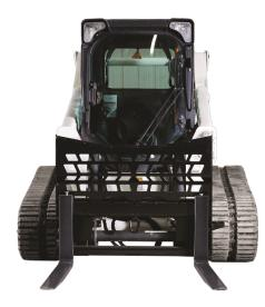
The Pallet Fork attachment is a vital tool for any industry where bulk pallets or palletized materials need to be moved. Just lift the lock and move them from 8" to 48" seperation. Also features a special D-Ring for securing loads with ease.
